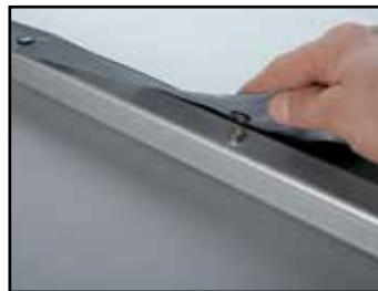
The elastic screen material is placed on the frame and attached to the frame via snap fasteners. The supplied legs are then fixed to the rear of the frame by means of wing screws.
